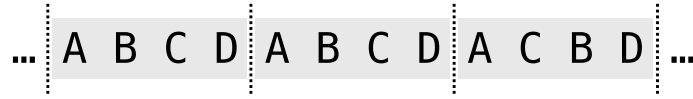
Figure 1.2: An example sequence of user interactions. Each character corresponds to a user interaction and the interactions are ordered based on their timestamp. Case attribution is the process of identifying those interactions that belong to the same process instance. Related interactions belonging to the same process instance are indicated separated by the dashed lines in the graphic.
